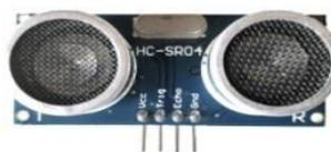
Fig. 2.6 Ultrasonic Sensor
