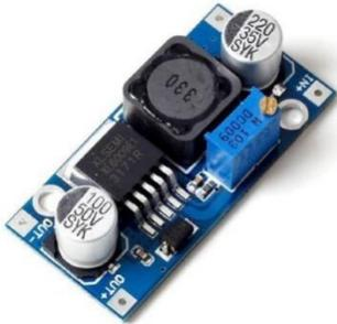
This is a buck-boost converter use for the equalization of the power coming from the solar panels. And it also safeguards the battery from the larger voltage and current.
